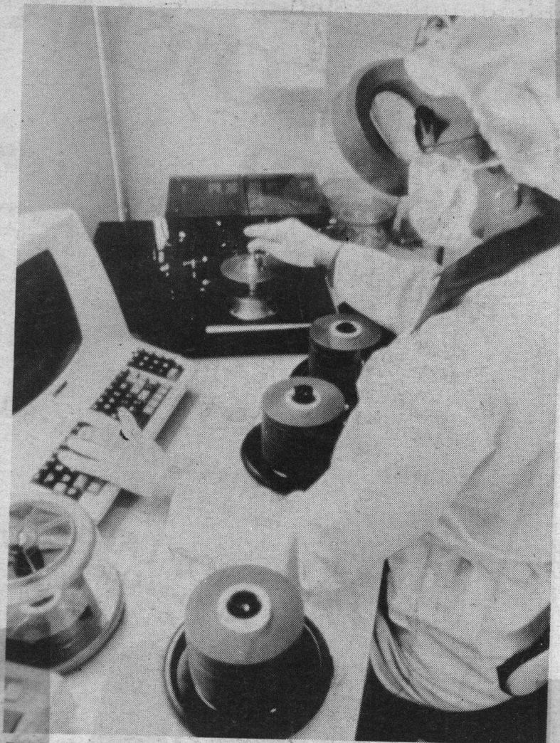
Rigid disk platters are tested for spin tolerance. As the surface of the platters must be free of all contamination, workers dress as if they're performing surgery.
