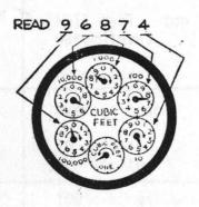
The second type of meter is the circular meter. The circular meter is read by noting the figures on the dials as shown in the illustration. When a pointer is between two figures read
