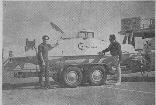
students are marine biologists. The subs run off batteries and engineers who use the subs which operate three to four the harbor. The one-man craft, for underwater structural in-hours without recharging. Air is spections and exploration.
