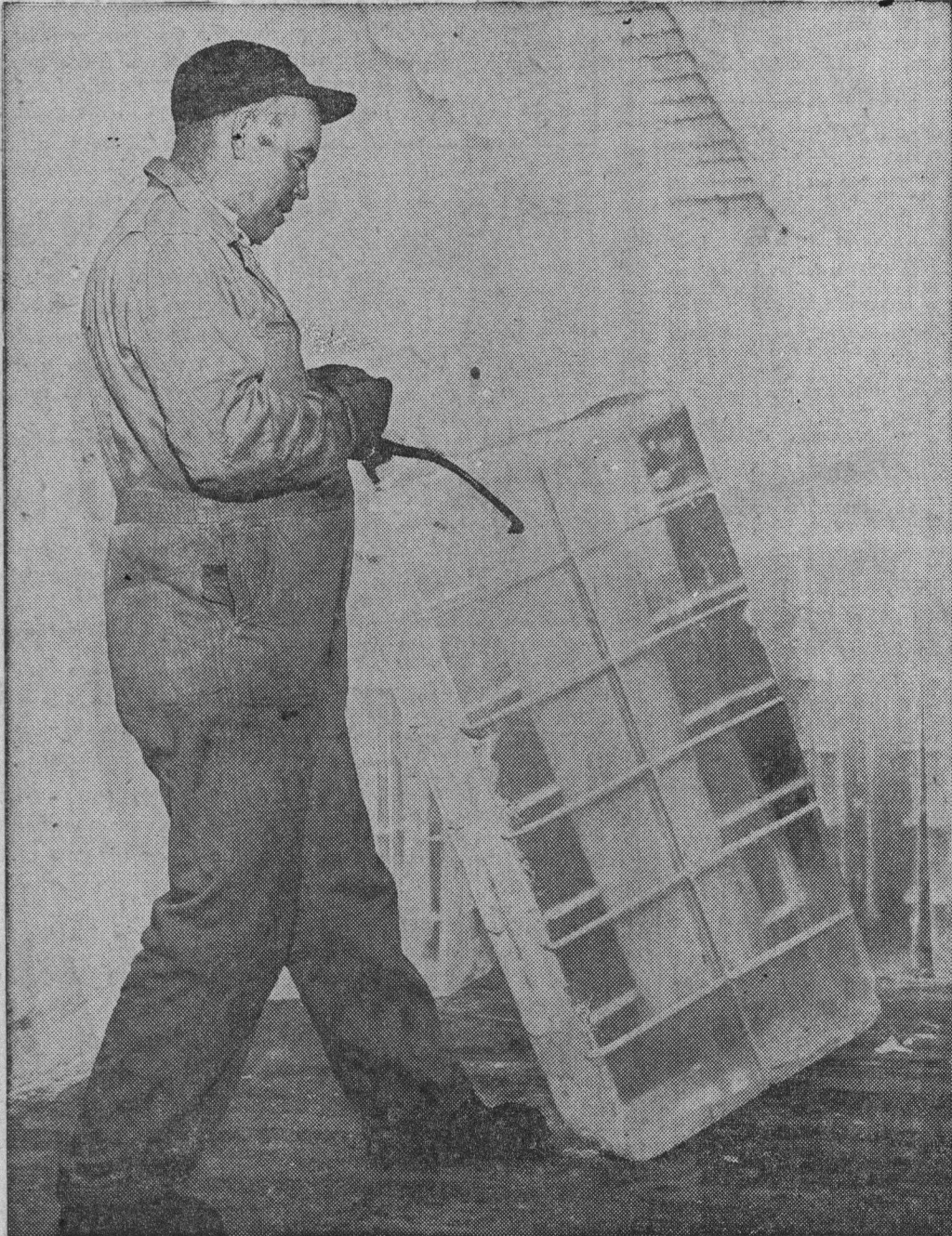
Darold Young muscled a 300-pound block of ice into line at the Union Ice company plant. Young, of 433 Cayuga street, said it takes 100 gallons of water to make the 40-gallon blocks. The remaining 60 gallons is
