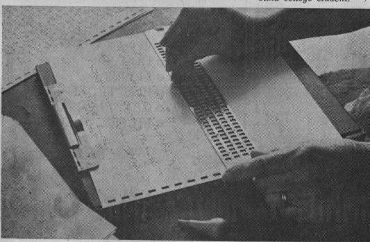
CORRECTING pages of machine-made dots is a by-hand process. Here Mrs. Naylor demonstrates the technique, with the page clipped firmly to the slate. With the stylus she is adding a dot that was accidentally omitted from the page. The little wood-en "eraser" lies on the
