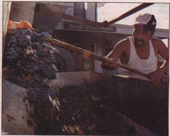
Melisio Leon Perez rakes grapes into a machine which crushes the grapes and allows them to release their juice.
